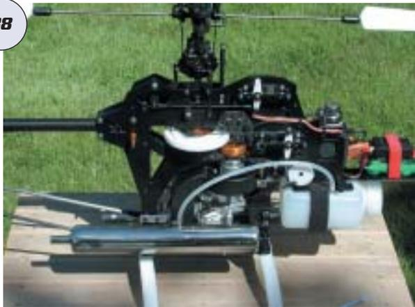
Neat and yet compact mechanical layout - no wasted space here. The Zimmermann 90-size muffler is an early example and has since been replaced with a later 2-piece version.
