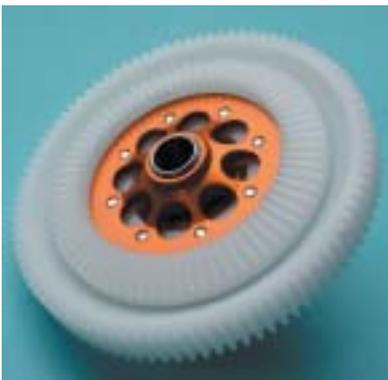
The auto hub is a one piece unit, the upper bevel gear carrier has a hardened sleeve (factory assembled) which protrudes down through the Torrington bearings. Make sure the gears fit perfectly flush on their base and tighten the screws evenly for a true-running assembly.
