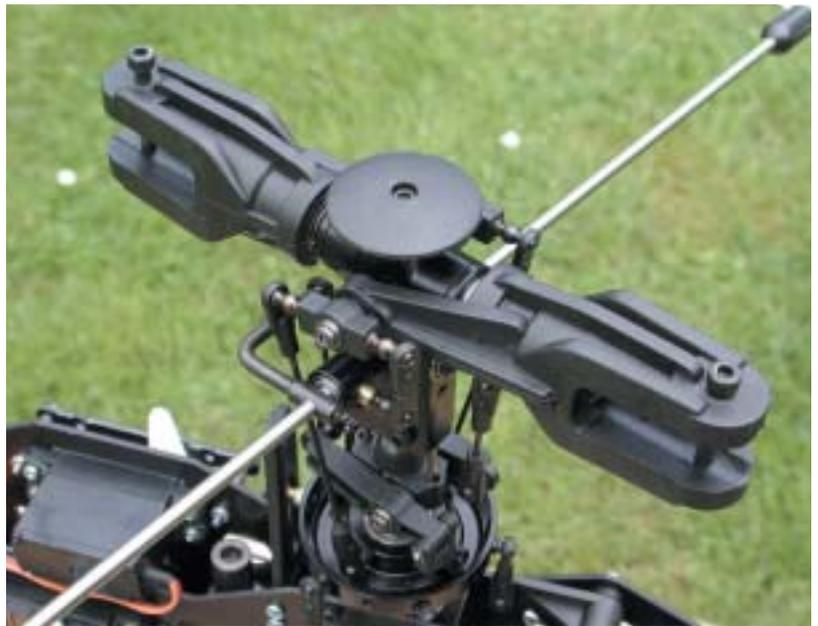
*This rotorhead works extremely well! The Flybar seesaw is machined aluminium as is the head block. Note the double ball ends used on the levers and flybar carrier so you can experiment with mixing ratios. 5 mm blade bolts are used. The washout hub is the GRP item as it's proven to be slop-free and as you would expect, all rotating parts are ball raced.*
