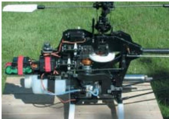
Large fuel tank gives good flight times. Note how all the servos are in line with their control rods and all the rods/bellcranks are at 90°/perpendicular - just as they should be at centre stick/0°. The flybar weight are optional and fully out as shown, give a nice feel to the model - Russ Deakin moved them in!
