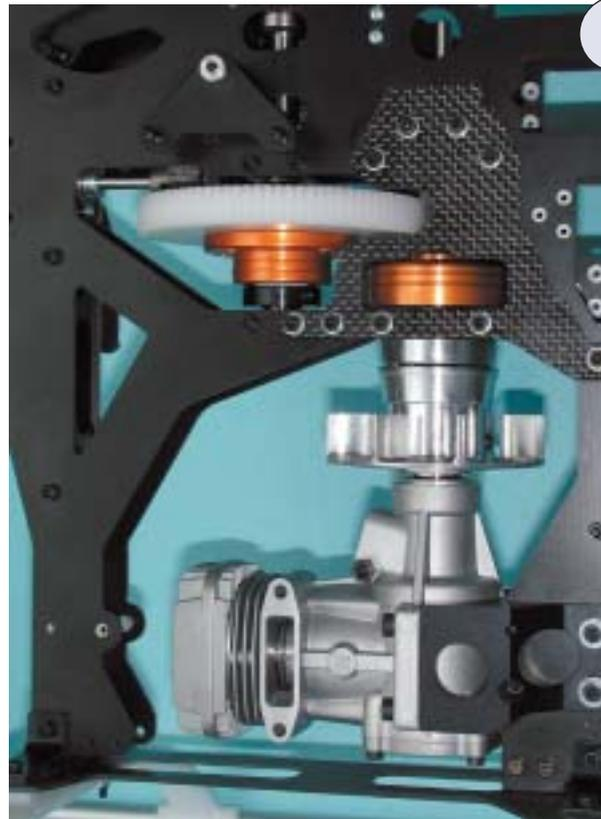
OS 91 with the excellent CNC cooling fan. The engine mount is a 3-piece affair. Note the carbon base plate is used to provide clearance for the larger engine. The upper carbon frame doubler is repeated on the other side adding strength to the high stress area.
