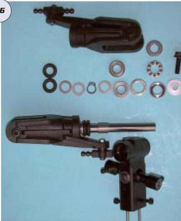
Here you can see the 8 mm parallel ground through spindle with 8 mm i/d thrust bearings. It has a piece of tube in the centre to provide centre support, with twin 'O' rings each side for teeter/feather damping. In the bearing line up, you see the 'O' rings, a selection of shims and then a circlip which locks into a groove on the spindle. This pre-loads the damping and allows the grips to rotate independently of the damping.
